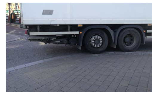
Figure 15-8 HGV mounting the footpath due to restricted capacity at the South Quay / Bridge Street Junction. Source: DBFL.
