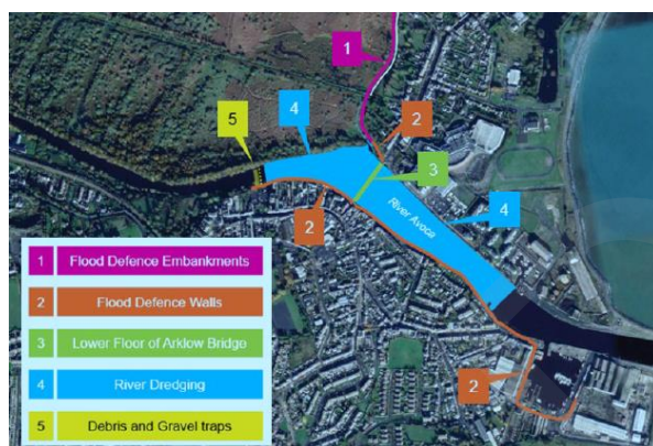
Figure 8-2 Scheme Aerial View. Source: Wicklow County Council.
